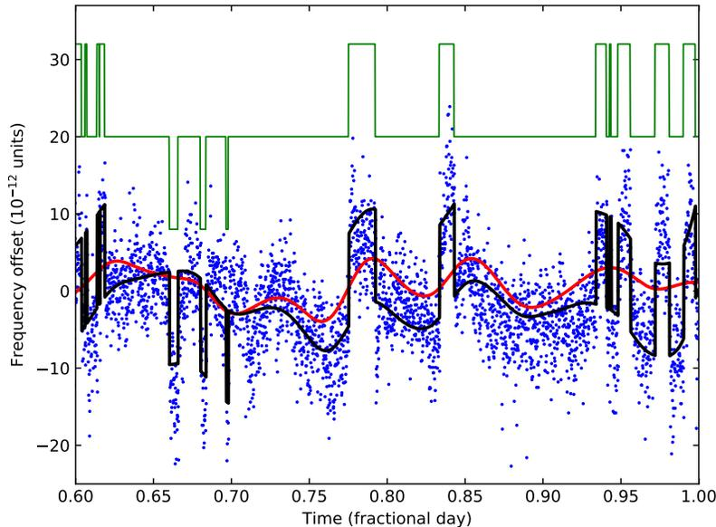
**Figure 4.** An example prediction result on a test data set (not part of the training set; same period as in Figure 3). The blue dots are UC measurements; the red thin line is the low-pass-filtered frequency offset; and the black thick line is the prediction result. In terms of error reduction, the mean squared error in the example is reduced from 71.5 (total UC variance) to 45.2 (post-fit variance), in units of  $10^{-24}$ .
