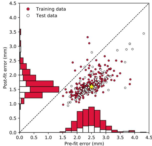
**Figure 5.** Comparison between pre-fit XL-DC clock structure and post-fit structure—expressed in millimeters as described in the text, having subtracted intrinsic variance from the Cs clock and universal counter. Each dot represents an individual 24-hour period. The diagonal dashed line shows where the pre-fit and the post-fit measures are equal. Points below the diagonal line indicate improvement. The star indicates that a typical improvement is from 2.5 mm to 1.6 mm.
