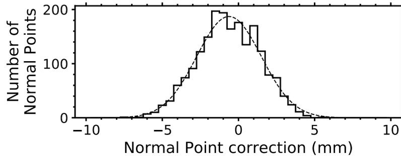
**Figure 6.** Corrections to historical APOLLO normal points based on the correction algorithm applied to GPS clock data, in 0.5 mm bins. We find an offset of  $-0.65$  mm and standard deviation of 2.0 mm (2.1 mm according to Gaussian fit).
