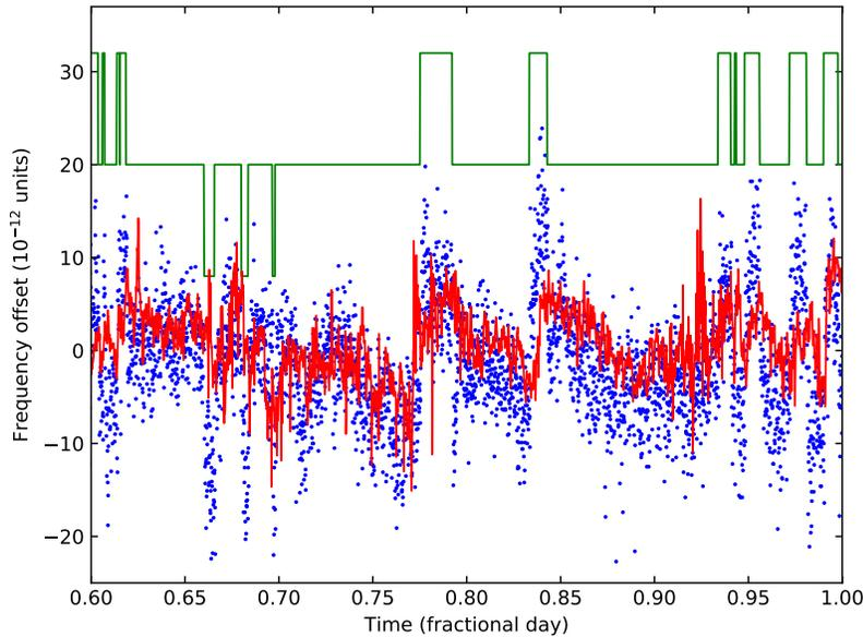
**Figure 3.** Comparison of XL-DC reported frequency offset (red jagged line) and DAC (green at top, offset arbitrarily) to the UC measurements of XL-DC frequency (blue dots). The goal of the algorithm is to use the offset and the DAC information to best approximate the UC data.
