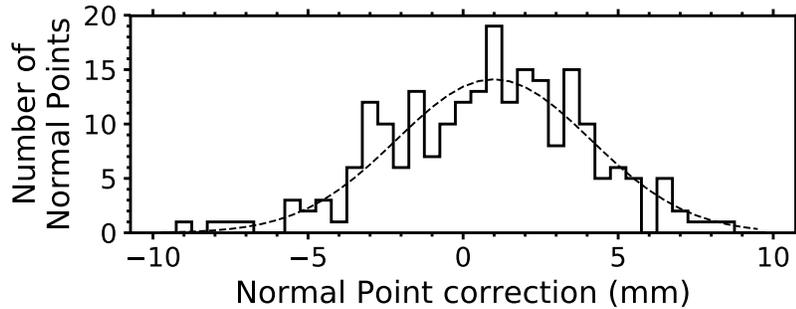
**Figure 2.** Corrections to APOLLO normal points acquired between 2016 Feb. 16 and 2016 December 12, in 0.5 mm bins. The corrections are based on the UC measurements of the GPS-disciplined clock offsets relative to the Cs clock. We find an offset of 0.9 mm and standard deviation of 3.2 mm (3.1 mm according to Gaussian fit).
